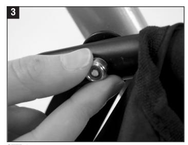
**STEP 3** - Attach the new nylon-lock nut by fingers only.
