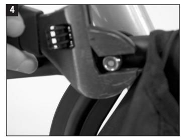
**STEP 4** - Use a wrench to tighten the nut until flush with the bolt end. Repeat this operation for the other side of the stroller.
