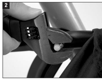
**STEP 2** - Remove the exposed nut by using a wrench.
