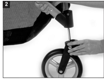
STEP 2 - Attach the new front wheel provided in the Repair Kit and push into the front wheel location until a "click" is heard. Tug firmly on the wheel to be sure it is securely in lace.
